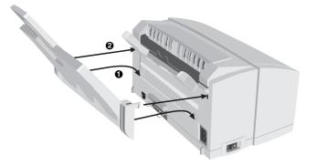
2 Push the paper tray forwards until it latches and is secure on both sides.
